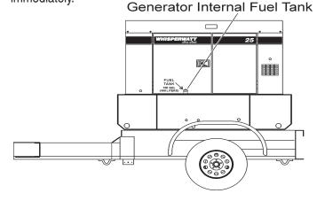
Figure 31. Internal Fuel Tank System
